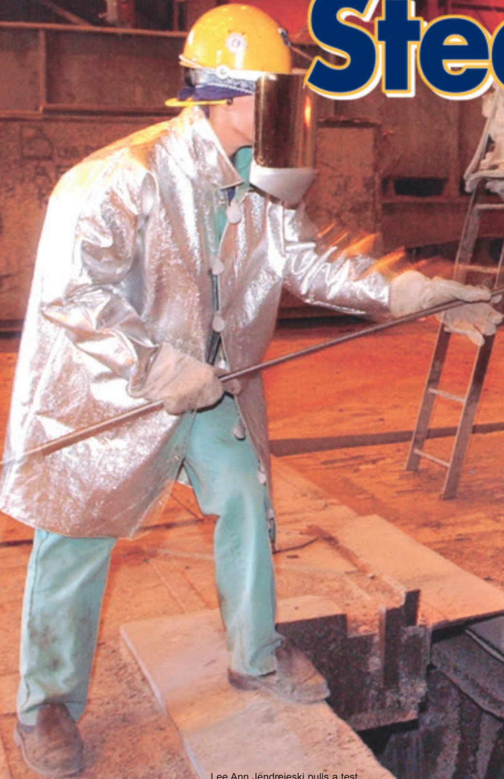
Lee Ann Jendrejeski pulls a test from an electric arc furnace at Allegheny Ludlum's Brackenridge, Pa. plant to check the chemistry of the heat.
